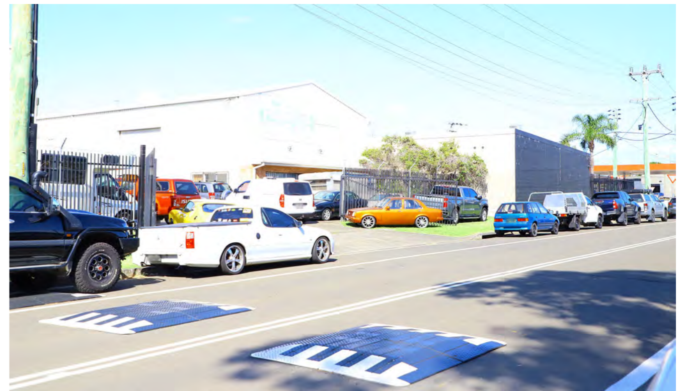
Figure 6.37: Illegal parking on verge and traffic calming cushions on Commerce Drive in Warilla Grove
