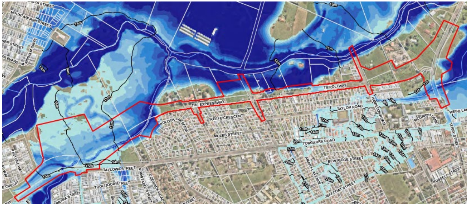
Figure 20: Existing 1% AEP Flood Extent
