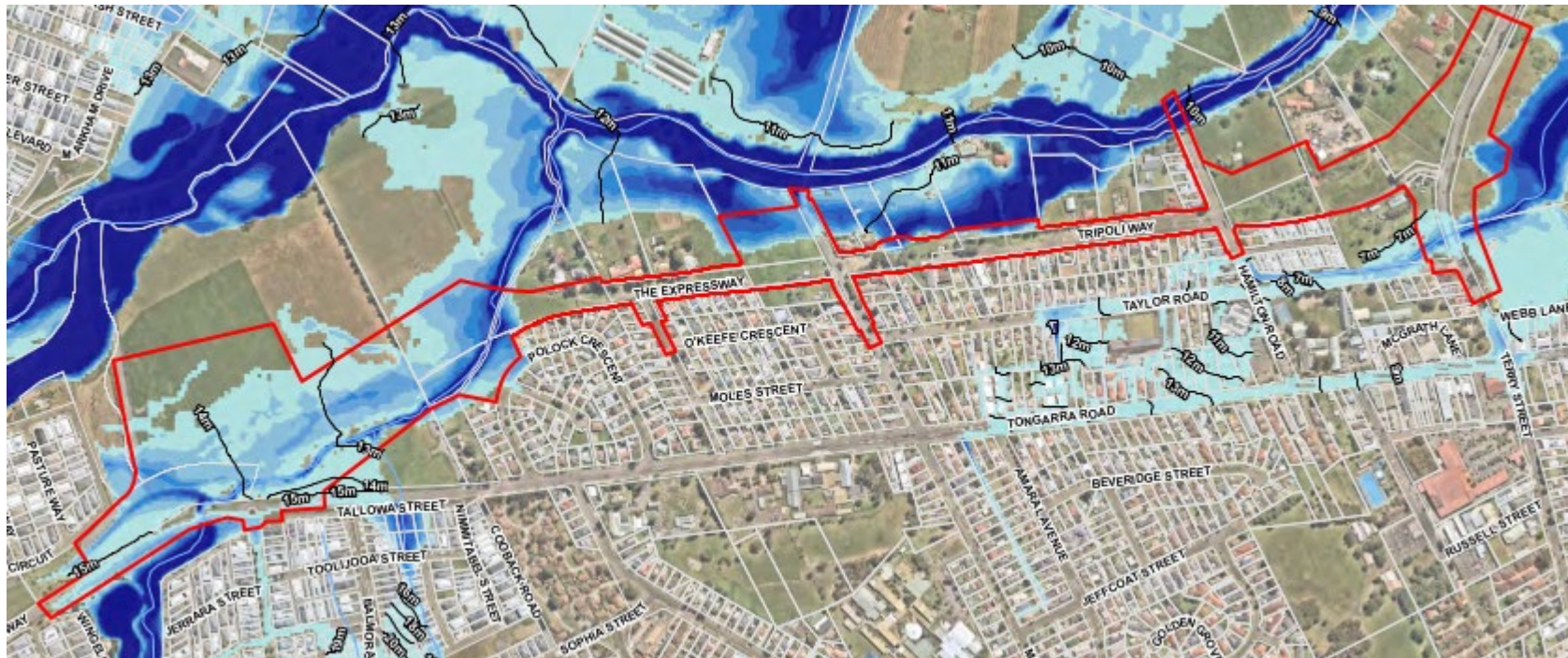
Figure 18: Existing 5% AEP Flood Extent
