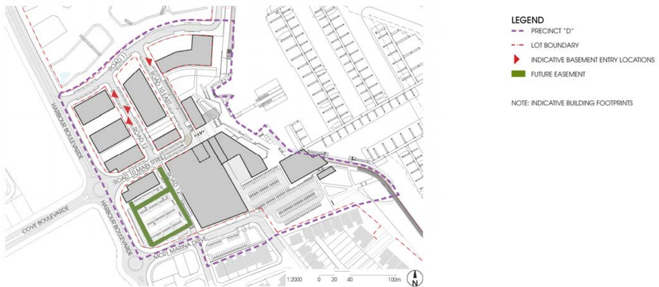
Figure 22 – Precinct D – Indicative Basement Entry Locations and Access Easement Source: Group GSA
