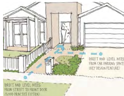
Direct and level access from street and parking areas (Source: Livable Housing Australia)
