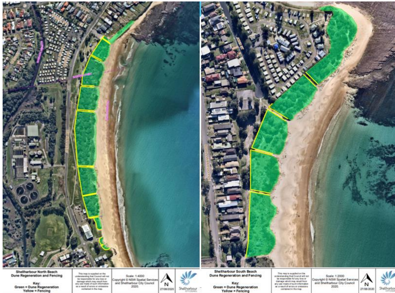
Figure 5: Dune restoration and protection works at Shellharbour North Beach (left image) and Shellharbour South Beach (right image). Green highlights indicate areas to be restored and yellow lines indicate fencing.
