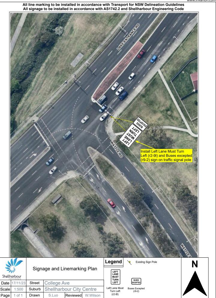
All line marking to be installed in accordance with Transport for NSW Delineation Guidelines All signage to be installed in accordance with AS1742.2 and Shellharbour Engineering Code
