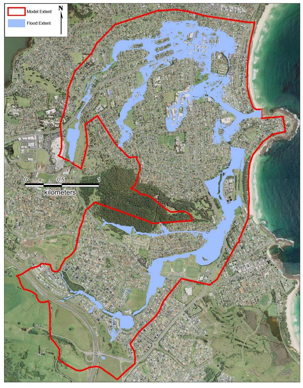
Figure F-4 Design Flood Extent for Existing Conditions – 5% AEP
