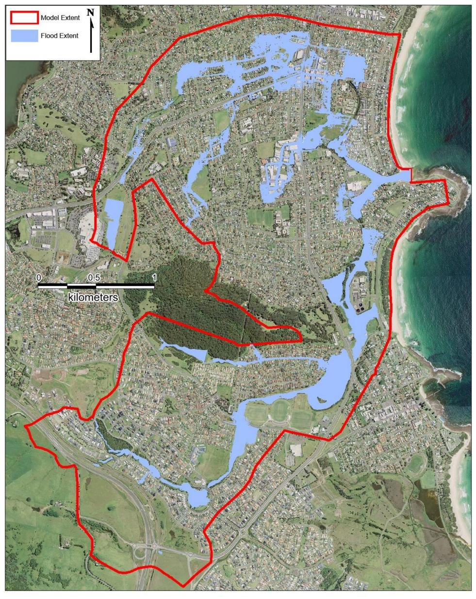
Figure F-2 Design Flood Extent for Existing Conditions – 20% AEP
