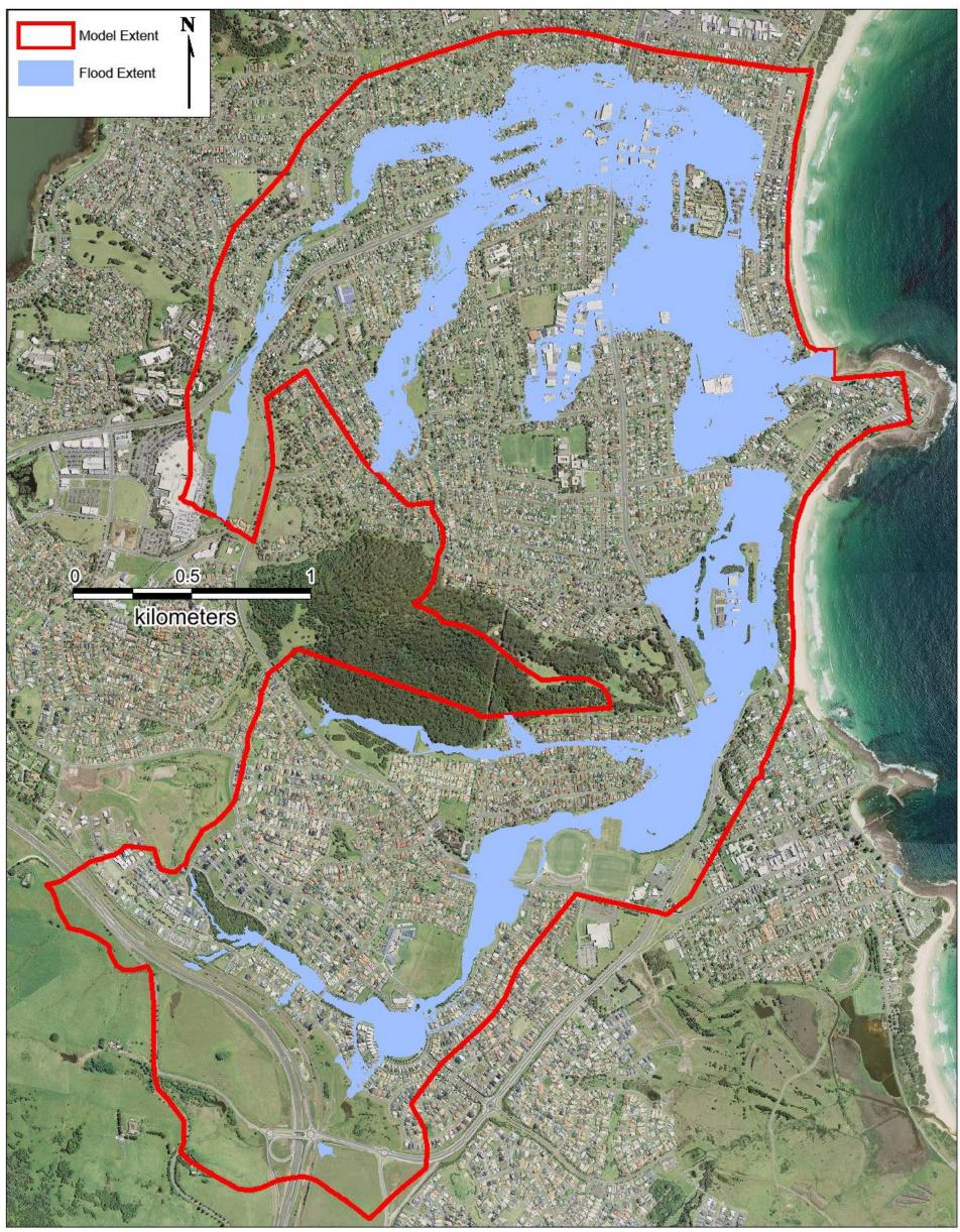
Figure F-7 Design Flood Extent for Existing Conditions – 0.5% AEP
