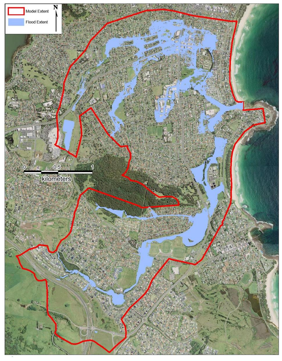
Figure F-3 Design Flood Extent for Existing Conditions – 10% AEP
